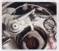
Set the points gap when they're fully open (at the highest point on the distributor lobe). Turn the engine by hand to get it to this point. On Lucas distributors, the points gap will generally be 15 thou.
