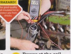
Applying that logic to engine electrics, if you've established the ignition switch is operational, check you're getting current from the battery at the coil by attaching a voltmeter to the coil's terminals.
