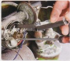
The points gap needs to be correct to ensure a good spark at the plug. Look up the points gap in your car's workshop manual, and use a suitable (and clean) feeler gauge to set it correctly.
