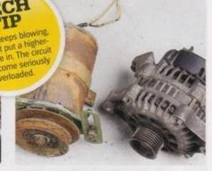
To make electricity, all you need is a conductor (wire), a magnetic field, and relative movement between the two. In a dynamo, the wires move around the magnet; in an alternator, it's the other way around.
