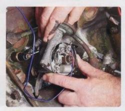
Now loosen its retaining screw and rotate the distributor housing (if necessary, crank the engine over to establish the correct direction of rotation) until you see and hear the spark formed when the points open. Tighten the screw again.
