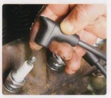
As the current goes to the distributor cap, the rotor arm sends it down the HT leads via contacts in the cap. It then arcs on the spark plug, igniting the fuel/air mixture.
