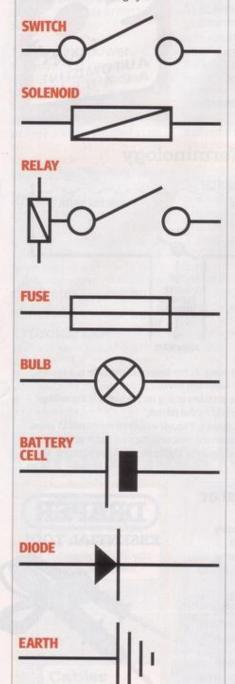
Don't be intimidated by the apparent complexity of a wiring diagram. Rather than trying to take in the entire thing, remember that you'll generally only need to be tracing one circuit or working with one part of it in order to either rewire it or trace a fault. To make life easier, the colour of the individual wires will also be given in the diagram.
