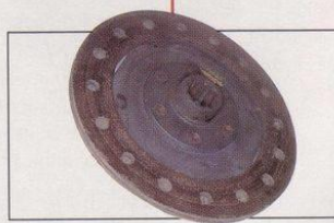
Driven plate: also called the friction disc or clutch plate, this is the sandwich filling. It's clamped between the flywheel and the pressure plate.
