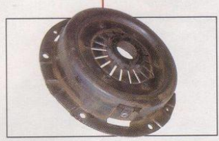
Clutch cover: second slice of bread in the clutch sandwich. Outer edge bolts directly onto the flywheel and a sliding pressure plate sits inside.
