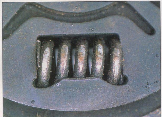
These torsional damping springs in the driven plate have been ground flat by contact with the flywheel or clutch cover.
