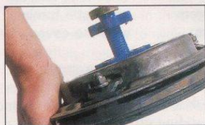
It clamps driven plate and clutch cover together, but struggles with heavy items.
