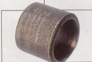
Pilot bearing: this sits inside the crankshaft. It supports one end of the gearbox shaft but allows it to turn independently of the crankshaft.
