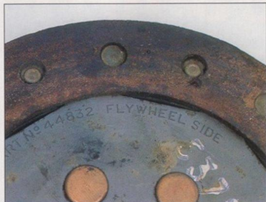
In a rare show of thoughtfulness, manufacturers make it impossible to fit a driven plate the wrong way round.
