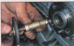
To shift it with an anchor bolt, you need room for it to expand beyond the bush.
