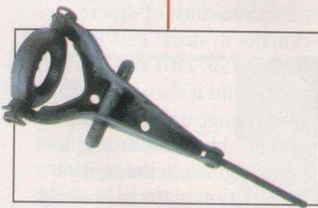
Release bearing: clutch pedal pushes the release bearing into the clutch cover. It can either turn with, or slip over, the rotating levers of the cars.
