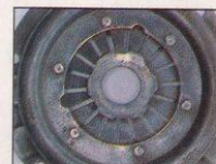
Here's a diaphragm clutch. This one has a central thrust washer to meet the release bearing.
