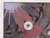
Red paint on fingers and white on the pivot point show how the fingers act as levers.
