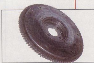
Flywheel: this is bolted directly onto the crankshaft, and is one slice of bread in the clutch sandwich. Outside teeth are turned by the starter motor.
