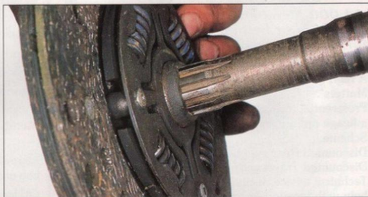
If the gearbox splines are rusty, the driven plate won't slide. Go sparingly with the grease, though, and don't use a general purpose grade.
