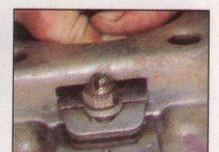
Push levers and they pivot like a see-saw, pulling pressure plate away from driven plate.
