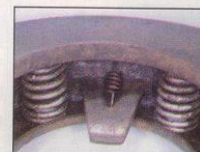
Inside, coil springs push a pressure plate away from the cover into contact with a driven plate.
