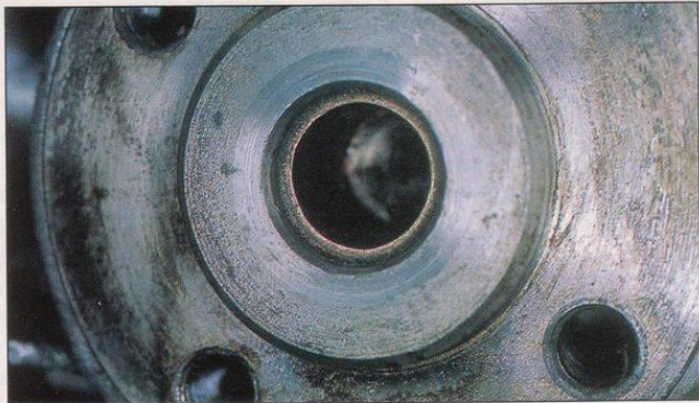
Worn pilot bush can cause all sorts of alignment problems.
