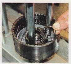
17 A pressing-tool like this is needed to push pistons in evenly. The top/reverse clutch, shown here, has a coil spring rather than a diaphragm, which has to be compressed to free its securing circlip.
