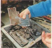
6 Usual reasons for dropping the sump between overhauls are to clean the main fluid filter inside (this one's unusually clean) or to renew the kickdown cable which attaches inside. Use new sump gasket on reassembly,
