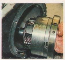
11 Then you can withdraw the main epicyclic gear assembly, followed by the annulus ring with the output shaft. Check for obvious damage and wear, inspecting teeth closely from all angles — they're usually okay.
