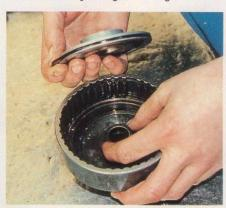
16 Clutch piston removal can be tricky as they're a tight fit. Using an airline on the other side is one way; another is to dislodge the piston by jolting the whole assembly face-down on the workbench.
