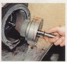
15 Next, slacken band adjustment right off (see picture 18), and then withdraw the pump from the front (picture 4), followed by the input shaft, complete with forward clutch assembly.
