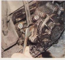
18 Now for band adjustment. Slacken locknut, then tighten centre pin to exactly 10lb ft and back off three-quarters of a turn (three flats). Then tighten the locknut down while holding the adjuster stationary.
