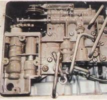
14 Before extracting the valve body carefully note exactly which pipes go where — as you can see, it is complex! The pipes pull out. You can then remove the block by undoing the  $\frac{1}{16}$  fixing bolts.
