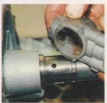
4 ...but the governor's fixed. Undo the locking bolt and slide the governor off. It fits on either way but must go back on with the small internal holes, of which one is visible here, facing into the box.
