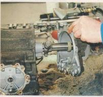
**9** At the back, remove the propshaft flange (one nut, very tight), then undo bolts holding tailshaft to main body, revealing spacer, speedometer drive pinion and the governor. Speedo drive and spacer bar slide off...
