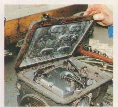
**5** You can drop the sump with the box in place — if the floor's clean! It's held by 12, 10mm nuts but you'll need a socket to reach them. Condition of fluid can tell you a lot — here it is water-contaminated.
