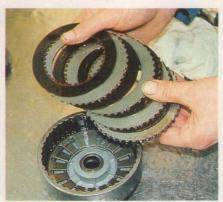
12 The 1st/2nd clutch assembly. Remove the circlip and take out the input shaft, followed by the clutch plates. The plates should be changed, as should the sprung diaphragm behind (forward clutch only).
