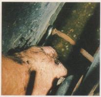
2 After dirty fluid, overheating is most common cause of autobox death. Many pass fluid through a cooler (underneath radiator) and pipes to and from it clog. Best, therefore, to renew pipes whenever 'box is changed.
