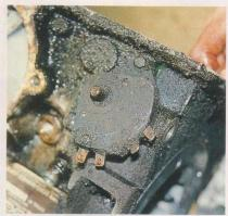
**3** You can change inhibitor switch yourself, although access can be awkward. A failed switch either stops car from starting in P and/or N or allows it to start when a gear's selected, which can be dangerous.
