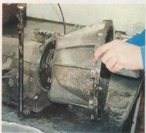
7 Stripdown starts with upending the 'box to drain out oil. Then take the bellhousing off (usually four bolts). It is also convenient to tackle the five 1/16 pumpfixing bolts (behind the bellhousing) at this point.
