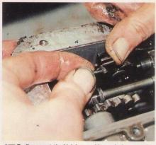
13 To disconnect the kickdown cable, push the operating arm forward and spring the cable inner outwards like this. The outer is a snap-fit and can be pushed up and out from inside using an appropriately sized socket.
