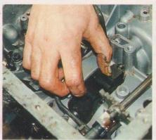
10 Once both clutch assemblies are out, pinch gear band ends together like this and push down so they too can come out through the front. Always fit new bands as a matter of course, they aren't expensive.
