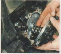
8 There are two external control servos, one on each side, each controlling one brake band. Undo bolts slowly and carefully — there's a spring behind and the cover may fly off. It can sometimes be difficult to undo.
